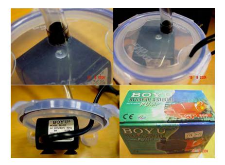
flowing back into the pail. It was then I started to notice that there are some air bubbles seeping into the container. It seems some air is seeping in through the inlet hole. Well, I proceeded to plug that hole with silicon to prevent leakage. The outlet hole was also given a coat of silicone for good measure as was the hole for the power cord to go through.
